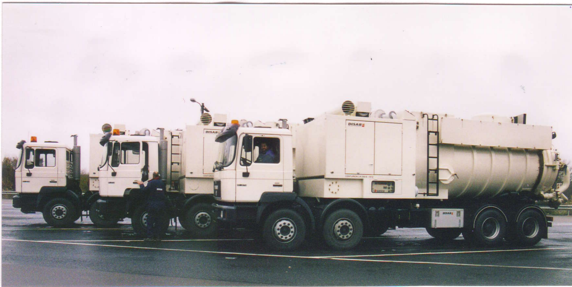
3 Nos. Vacuumloader with 230 kW dieseloperated vacuum machine, delivered to Baghdad Mayoralty, Baghdad, Iraq 1998.
